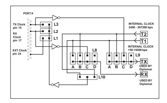
The following diagram illustrates the synchronous clock selection.
