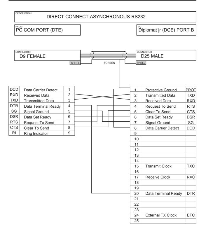
**Note:** It cannot be assumed that unlabelled pins can be used and no connections should be made to them.
